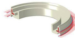
Fig. 14. Normal Stress vector plot
